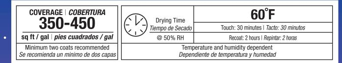
Modern MastersTheme Paint Exterior Dead Flat Varnish is a low VOC. 100% acrylic. nonvellowing, water base, protective clear top coat formulated with maximum levels of UV Blockers and UV Absorbers to further reduce the effects of harmful ultraviolet rays. It's clear, dead flat finish will eliminate any undesired sheen variations on the painted project. Not recommended for use over *Metallic Paint Collection*™ paints or Metal Effects ® oxidized finishes.
